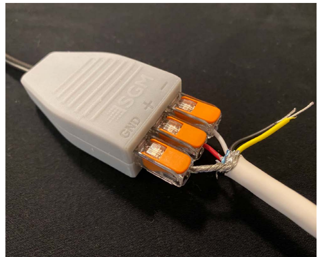
Figure 12: Connecting data to USB up-loader cable for POI fixtures
